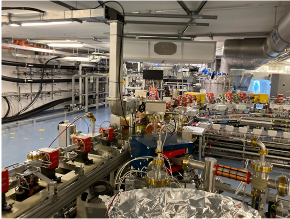
View from the injector line beam-dump towards the SRF photo-injector: Ready for beam commissioning
