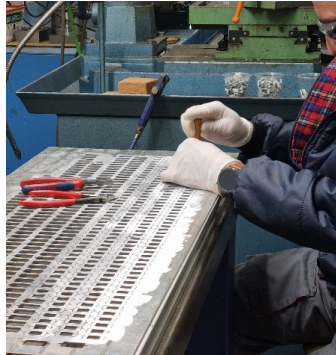
Mechanics fabrication 250 Minicrates ( 2 meters long) + 800 different pieces
