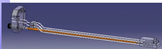
Patented RF ion source for compact cyclotrons
