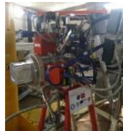
Sirius Silicon detectors used at GANIL/Spiral2-S3
