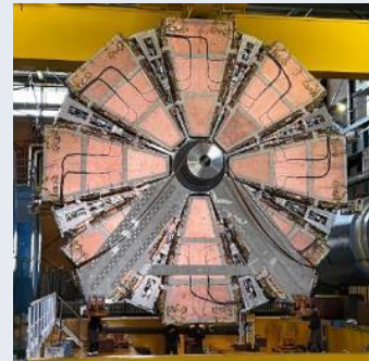
ATLAS New Small Wheels 400m 2 of Micromegas detectors
