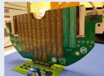
ALICE Muon Forward Tracker based on MAPS technology
