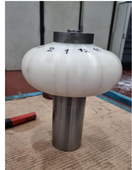
New 1.3 GHz Die for Spinning produced by Piccoli
