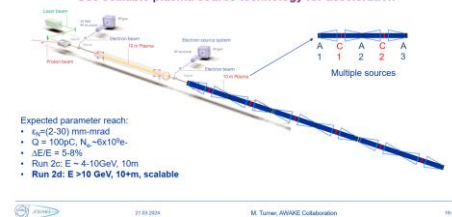
Run 2d: demonstration of scalability Use scalable plasma source technology for acceleration
