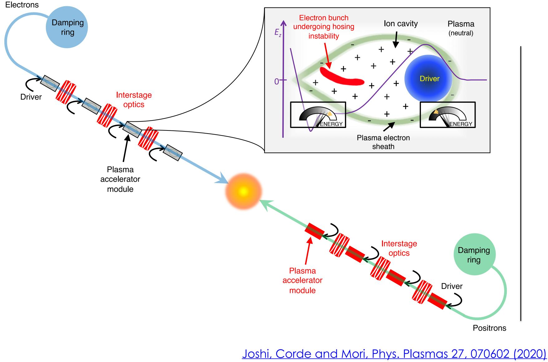
The blowout regime has ideal field properties for e-: emittance preservation is expected to be achievable. beam loading allow for high efficiency, flat  $E_z$  field and therefore low energy spread. most studied regime for electron acceleration, in both LWFA and PWFA. But: hosing instability may be an important limitation for collider beam parameters. ion motion may lead to emittance growth. what abut e+?
