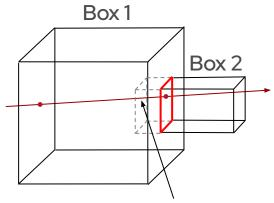
Missing the overlapping entering surface leads to missing Box 2 entirely
