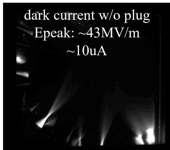
Dark current of the 2 nd gun, without(left) or with plug in(mid), and after re-processed
