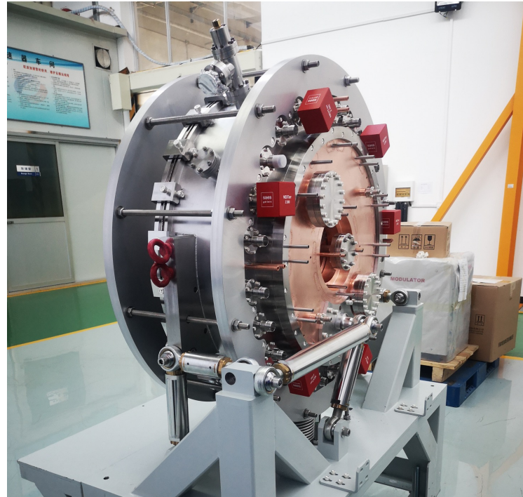
Gun 2 and 3, >75\text{kW} CW stable operation (limited by power supply system) with low dark current
