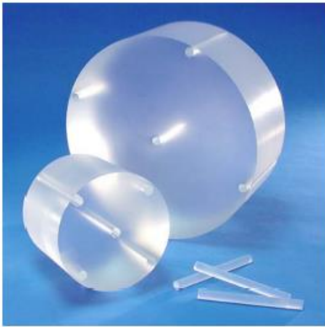
Phantom for CT made from plaxiglass
