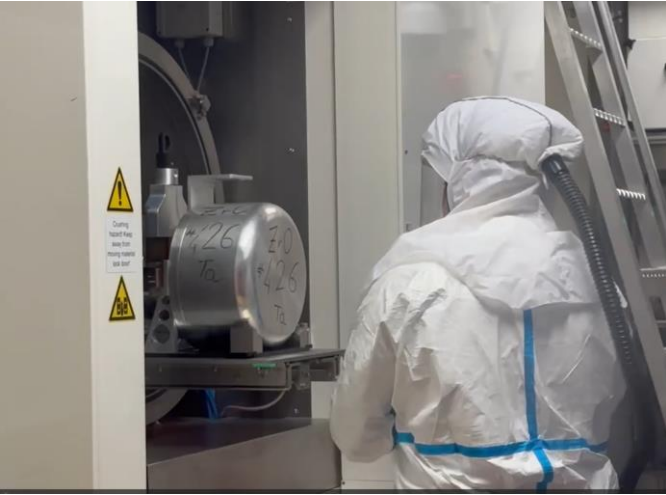
Drum filling (view from inside the hotcell)
