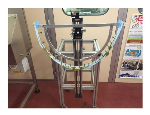
Should follow the loaded HR for testing, transport and insertion in the HS
