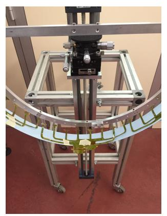
Addition frame needed to position the horizontal bar 10 cm below the micro-stages to avoid clashing with tilted table during HR pick-up.
