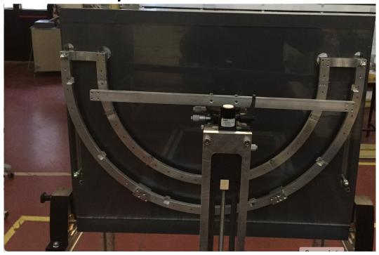
At this stage Fix HR inner arcs on integration tool by the horizontal bar
