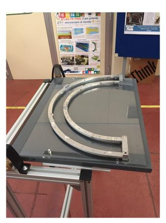
Remove upper HR End Pieces and fix HF outer arcs using its two M8 holes
