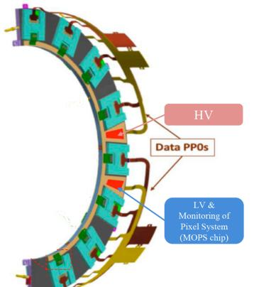
The PP0 flex is installed on the HR before integration and it is secured to the handling frame outer arc.
