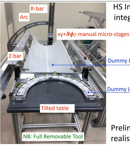
HS Integration tool positioned for the HR integration at LNF with HR insertion tool
