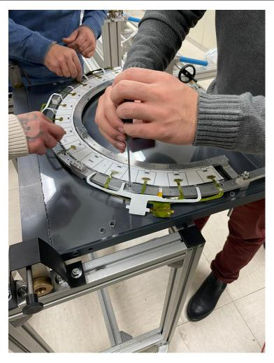
Remove lug clumps from HF outer arcs and free HR from HF outer arcs.
