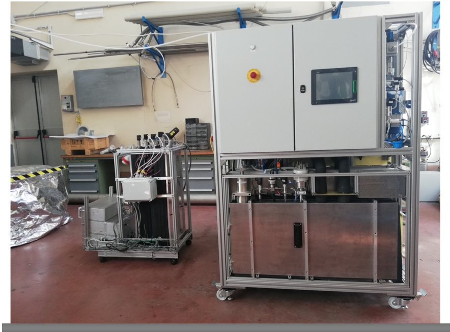
CO 2 Lucasz commissioned plant a LNF To do : Merging of lines from master and slave boxes to reach 20 g/s
