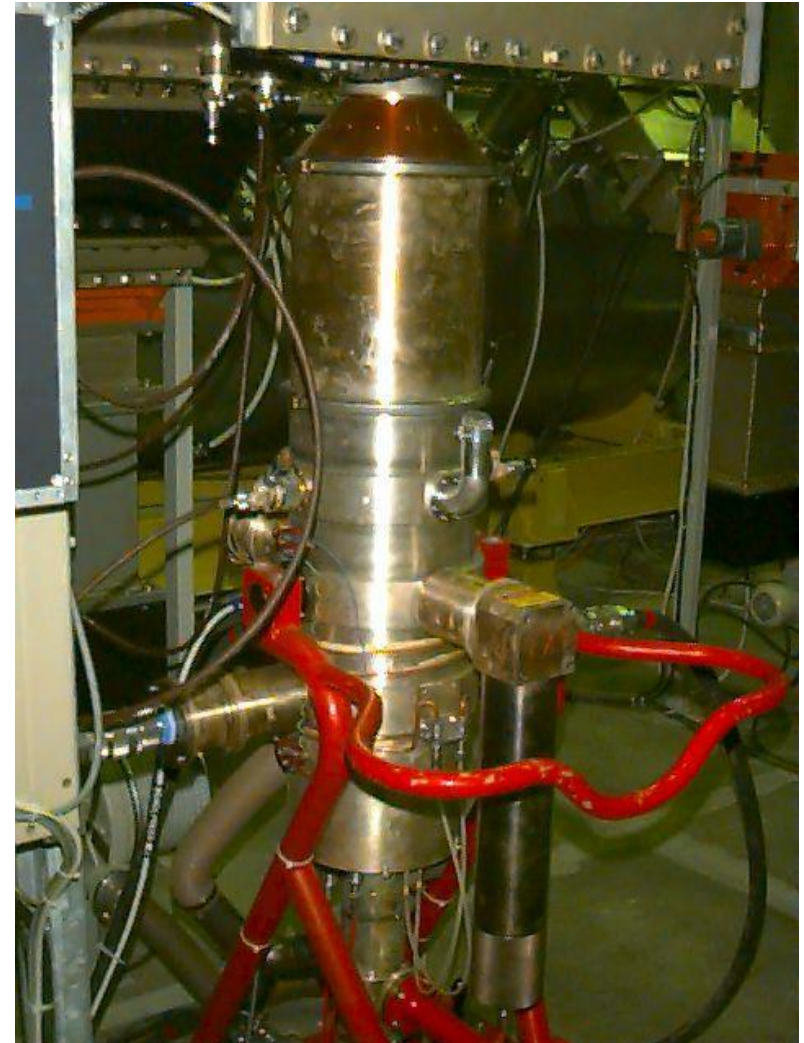
SPS 400 MHz Tetrode Amplifier
