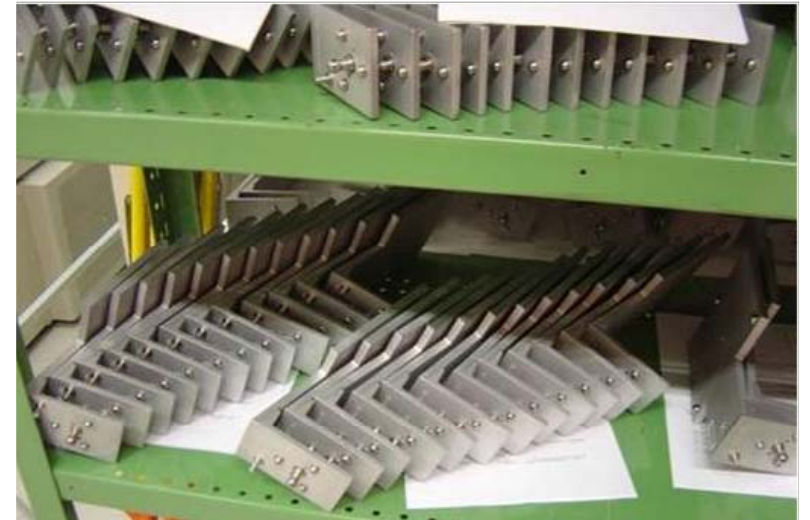
Extension plates with: 4 positioning spheres + pos. pin (sensor side) 3 positioning spheres (chamber side) (measured on CMM)
