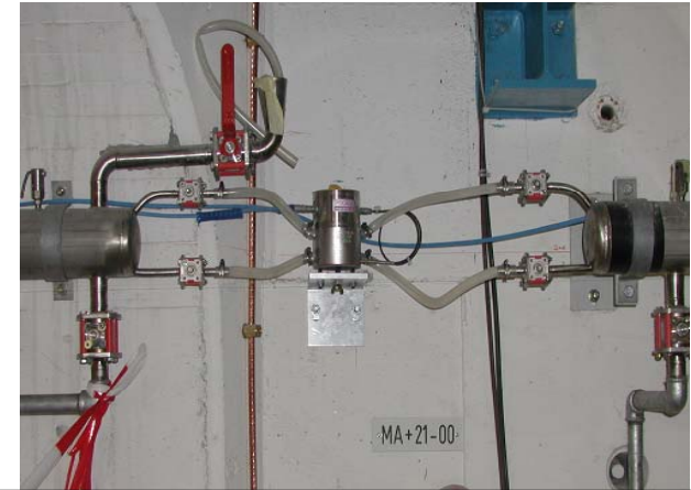
Machine HLS station system in the cavern (Atlas)
