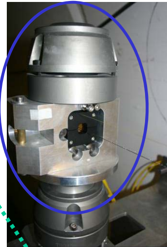
Machine HLS station system in the cavern (Atlas)
