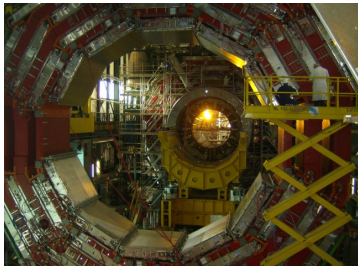
Muon detector: track sees 18–45 layers: an independent tracking system in its own right
