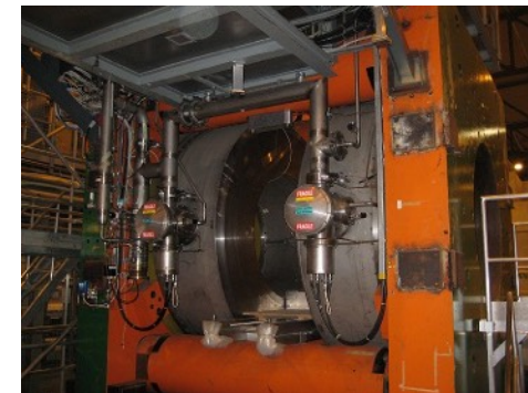
M1 SC Helmholtz coils at CERN H2 (3T)
