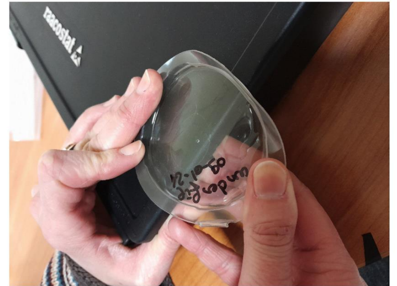
Requires re-curing at 80 C
