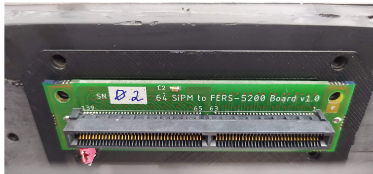
Front end board housing 64 SiPM
