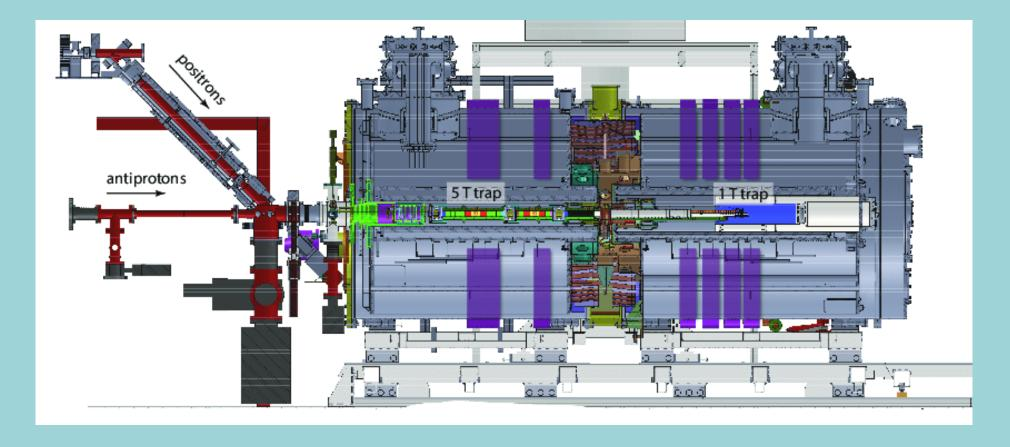
Magnetic system for anti-proton trapping in AEGIS (millions of antiprotons!)
