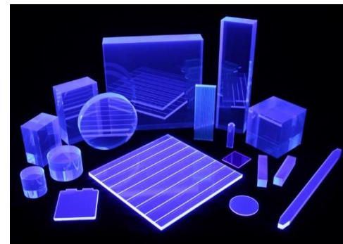
Plastic scintillator (+ fiber)
