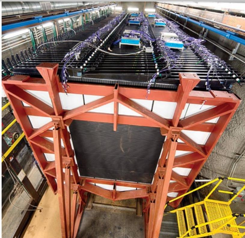
Far Detector: 14 kt,  $\sim 16 \times 16 \text{ m}^2 \times 60 \text{ m}$
