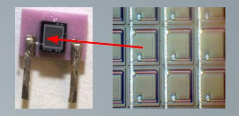
Overlaying SiPM signals cluster around 'integer' pixel discharges
