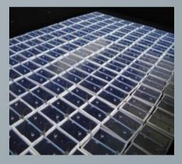
• SiPM: insensitive to magnetic fields, highly miniaturized, high gain (10<sup>5</sup>), low supply voltage (40V), plain wiring
