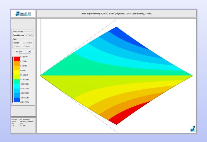
ASU Deformations (in direction z) of ½ PCB-wafer Max deflection was 0.21mm
