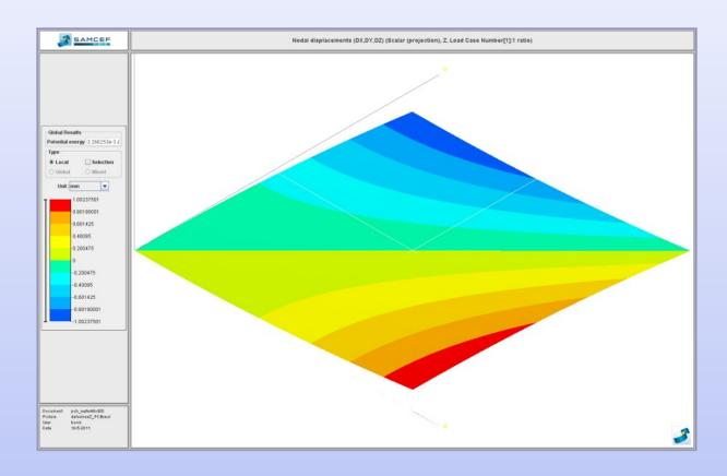
Deformations of ¼ shell PCB (2 symmetries applied). Maximale Deflection was 1mm.
