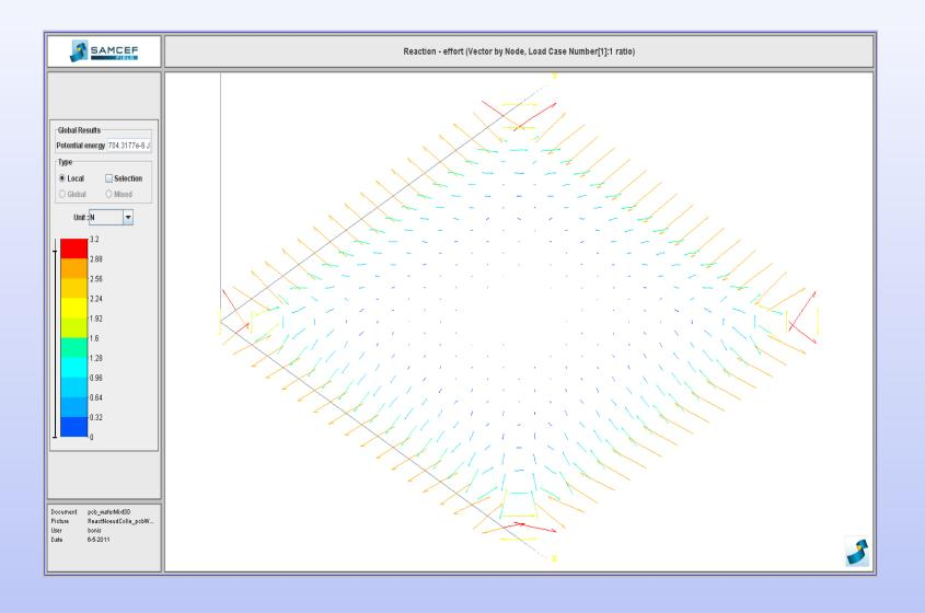
Node reaction in glue points (equivalent pads positions)
