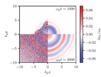
Clustering leads to small-scale perturbations of plasma density and transverse fields that can spoil the quality of accelerated beams and lead to early breaking and chaotization of the wave.
