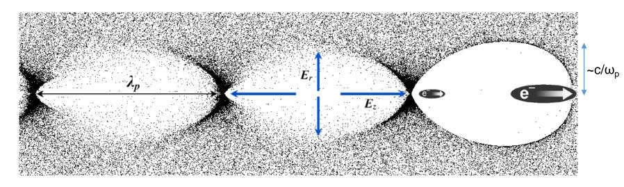
Electron temperature ~ 5 eV Electron thermal velocity  $v_t \sim c/300$   $\omega_p$  Debye length  $r_d = v_t/\omega_p \sim (c/\omega_p) / 300$ If we resolve  $r_d$ , then simulation time increases  $300^4 \sim 10^{10}$  times (3d PIC) or  $300^3 \sim 3 \cdot 10^7$  times (3d QSA)
