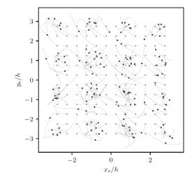
(Apparently) because we do not resolve the Debye radius in wakefield simulations, the macroparticles are attracted to each other, forming clusters and heating up.
