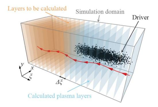
Quasistatic "macroparticle" is a "string" composed of real particles that enter the simulation domain at different times but at the same transverse coordinate and with the same initial momentum
