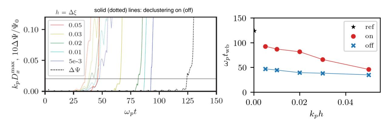
As the grid step decreases, the wavebreaking time approaches that observed in the reference run, but only when the declustering is enabled. If not, then the noise provokes earlier wavebreaking for any resolution.
