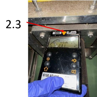
Dose rates (mSv/h) measured Nov 2023 around target (left/center) and at contact with CNGS target collimator (right)
