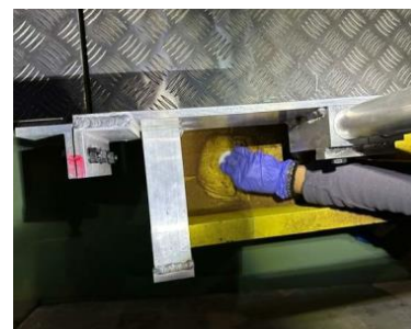
Surface contamination measured Nov 2023 at target table and at CNGS target collimator (right)
