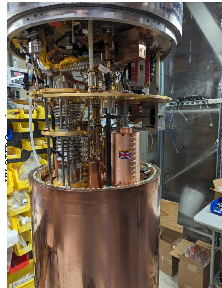
ADMX detector with UK sidecar cavity installed, ready for cooling. December 2023.
