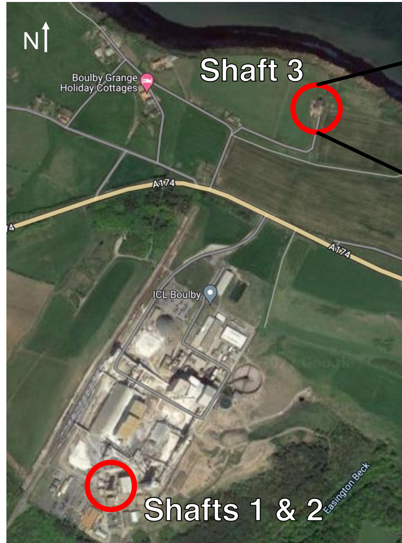
Shaft 1 & 2 (depth-1.1 km): Deep access shafts Shaft 3 (depth-180 m): Tailings Shaft
