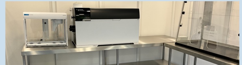
ICP-MS (Surface): Newly installed system for trace element analysis and isotopic ratio measurements.
