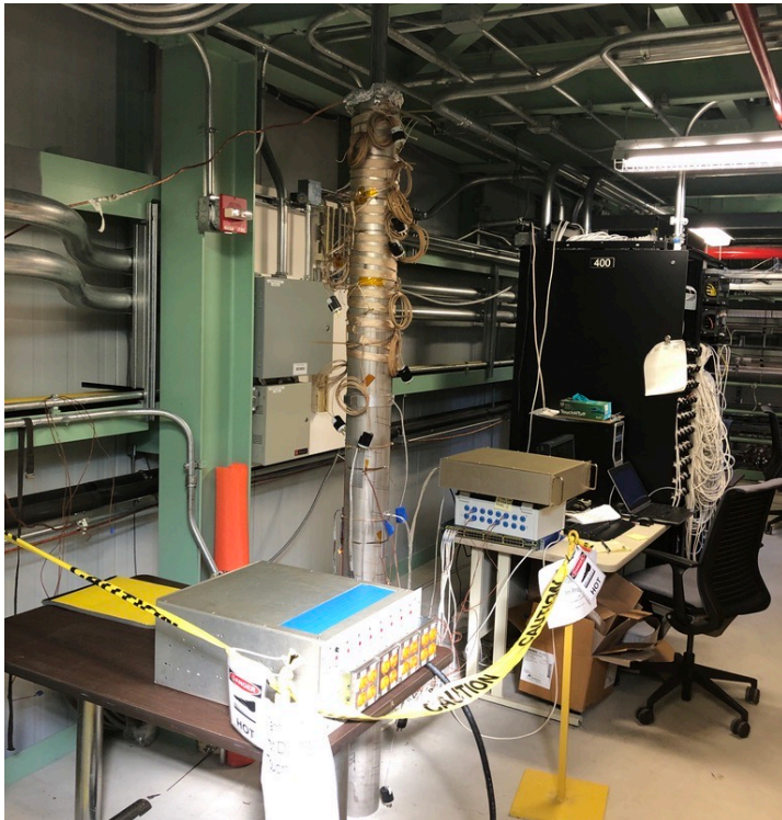
16-channel bake test setup.
