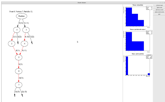
Figure: Pythia 8.2.40 simulated process e^+e^- \rightarrow \tau^+\tau^- with ISR and w/o hadronisation and decays. The display shows event information (e.g. run and event number, ...), depicts vertices as ellipses and the particles as arrows. The information on vertices and particles (ids and flavor) are given as well. The right panel shows selected distributions of physical quantities in the event, e.g. transverse momentum.
