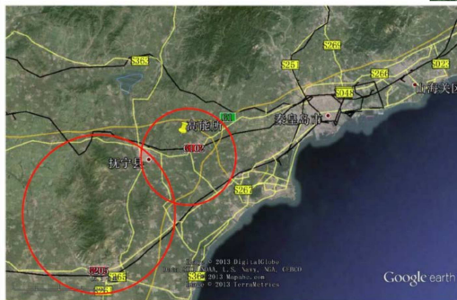
Figure 3.3: Illustration of the CEPC-SPPC ring sited in Qinghuangdao. The small circle is 50 km, and the big one 100 km. Which one will be chosen depends on the funding scenario.
