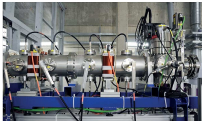
The accelerator used to produce fast neutrons. Image credit: SCK•CEN. Used by permission.
