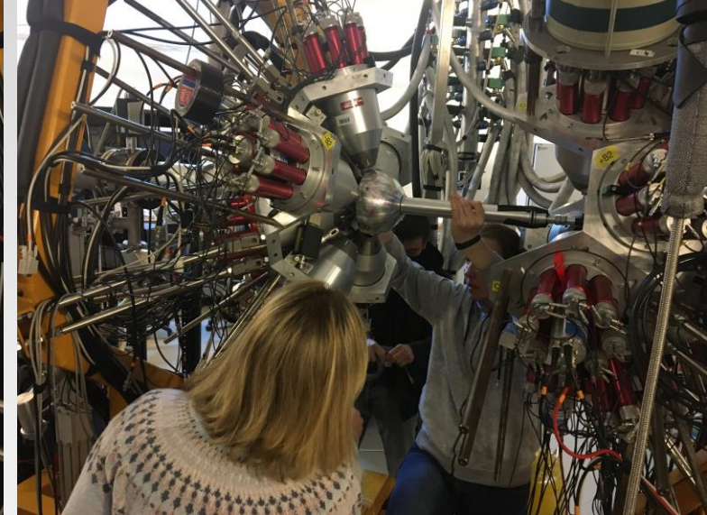
A setup for high-energy \gamma -ray spectroscopy with the ELI-NP large-volume LaBr 3 :Ce and CeBr 3 detectors at the 9 MV Tandem, S.Aogaki et. al., Nucl. Instrum. Methods Phys. Res. A, 1056, 168628 (2023)
