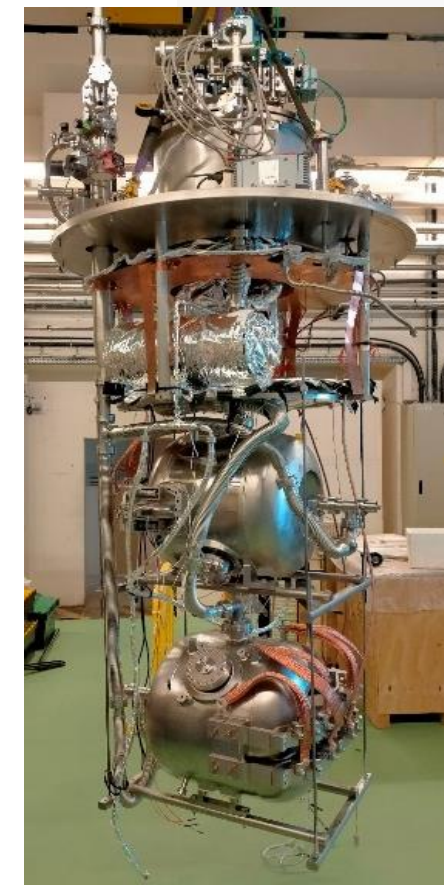
PIP-II Spoke resonators built by Zanon installed on insert 7
