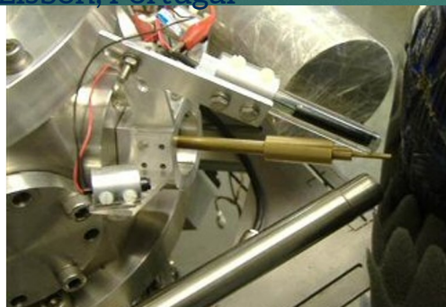
nuclear microprobe @ 2.5 Van der Graaff accelerator and external beam
