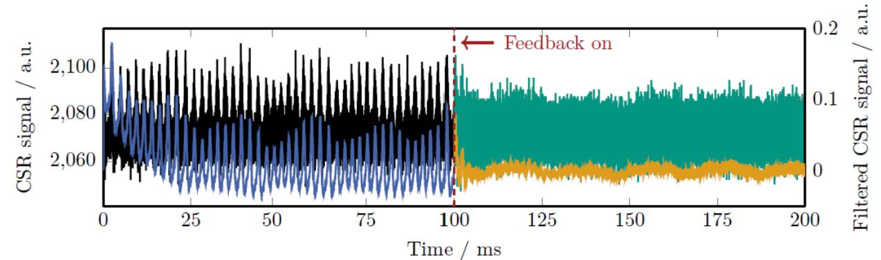
The CSR signal was measured with a fast Schottky diode (at a KIT infrared beam line).
