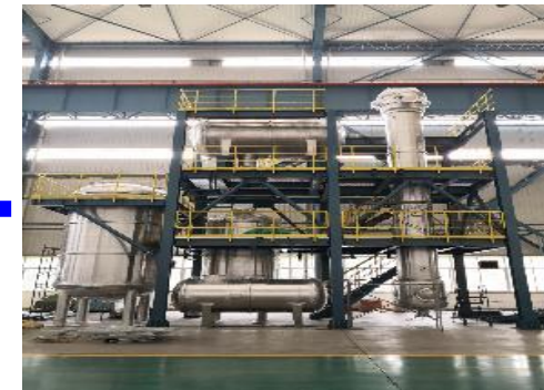
3) Water extraction to remove radioactive impurities
