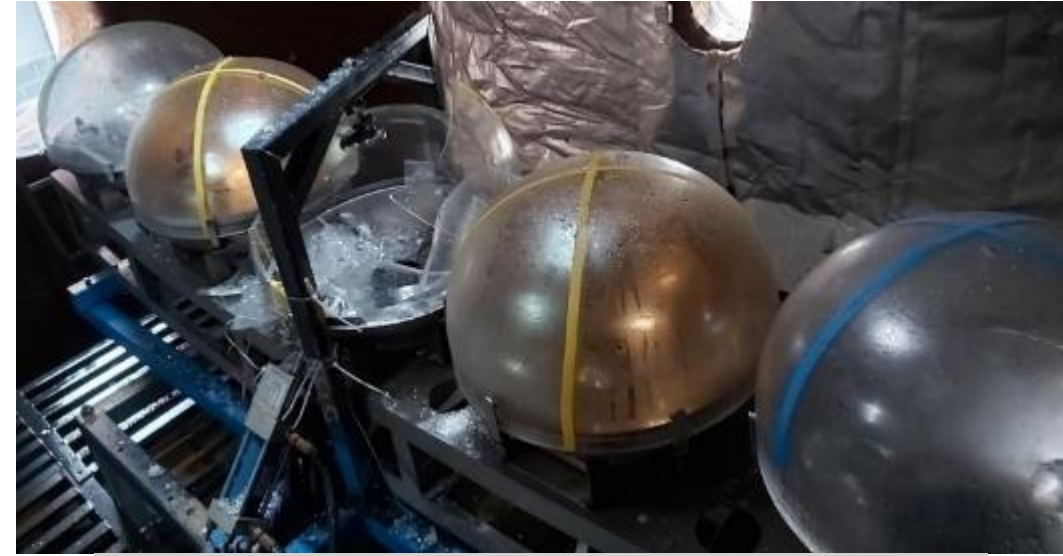
Implosion test of PMTs on the module structure
