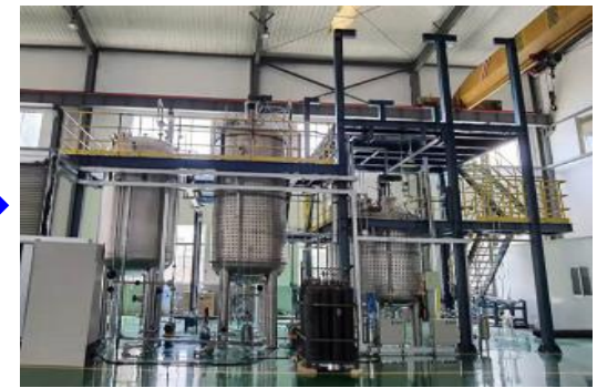
Mixing LAB with PPO and bis-MSB
