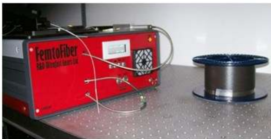
FemtoFiber + scanning head for confocal/2PF imaging = FiberScope
