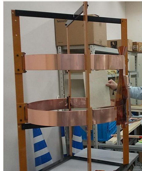
Real scale prototype of kicker coils
