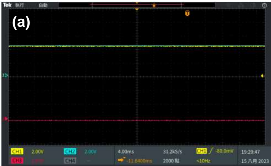
(a) Output of the preamplifier without applying the high voltage for the two-output channel is shown in blue and yellow, whereas the signal inhibit is shown in red.
