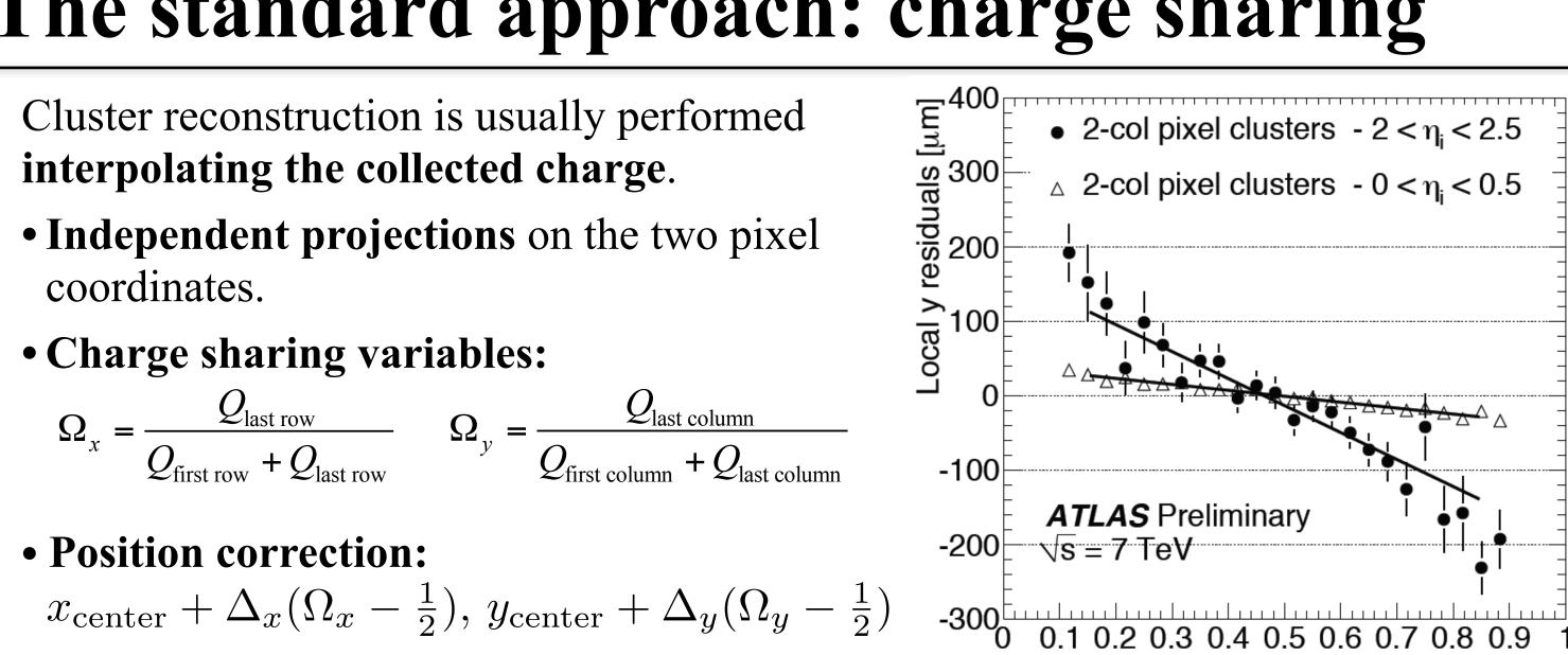
ATLAS Preliminary  $\sqrt{s} = 7 \text{ TeV}$ residuals 30 25 × local 20 of RMS Center of the cluster Charge sharing algorithm Track incident angle  $(\phi)$
