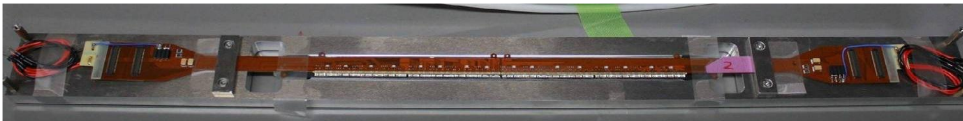
Pixel stave (with cooling)
