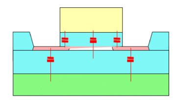
Cj is 1/10 of Bulk technology. Gate Capacitance is 30-40% Lower.
