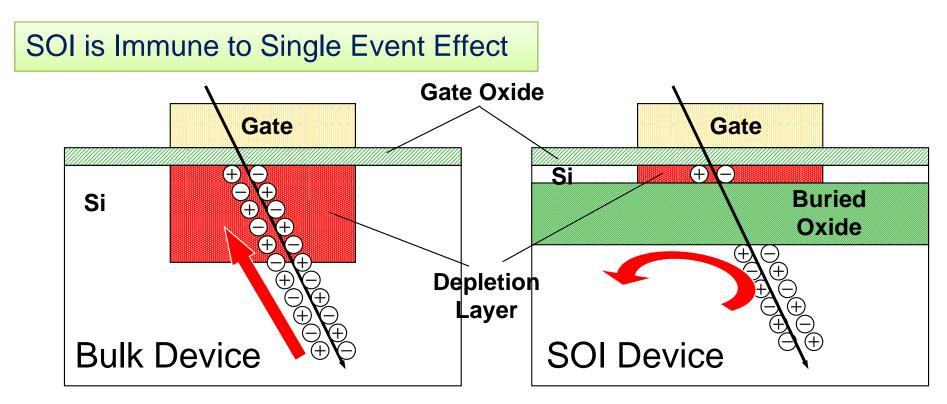
But not necessary strong to Total Ionization Dose due to thick BOX layer
