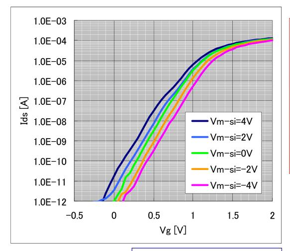
Nch Core Normal-Vt L / W = 0.2 / 5.0 um Vd=0.1V, Vback: floating Threshold voltage of a transistor is controlled with the bias voltege of the Middle-Si layer. This indicate effects of the trapped charge in the BOX can be compensated with the bias voltage.
