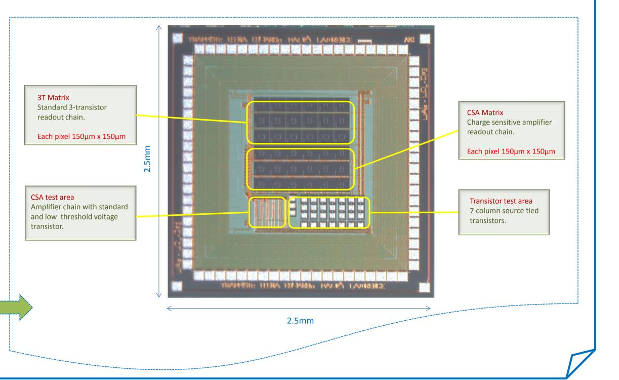
Challenge: Its use is subject to the back gate effect because of the voltage applied to deplete the detector. Solution: Among others, increasing the oxide thickness and including different well implantations below the read-out circuitry.
