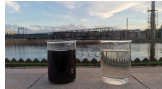
Comparison of wastewater before (left) and after (right) electron beam radiation. (Photo: Nuclear and Energy Technology Institute, Tsinghua University)
