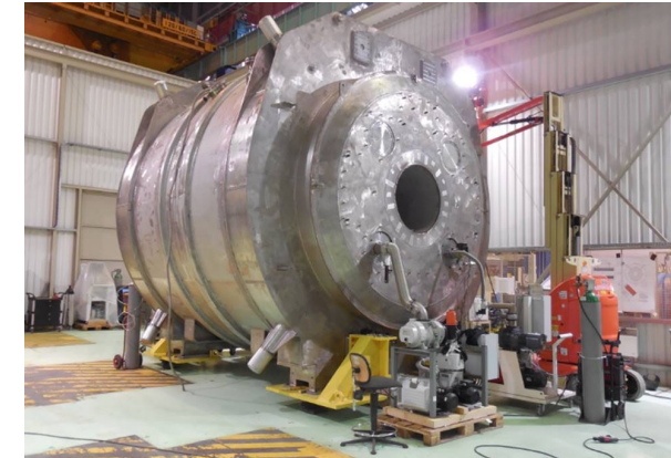
UHF MRI magnet (11.7 T, 900 mm bore, full body) developed by CEA/Alstom
