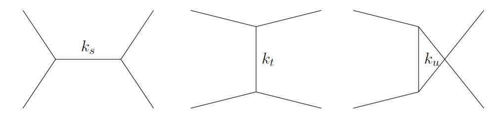
$$\mathcal{A}_4^{\phi^3} = \lambda^2 (2\pi)^d \delta^d \left( \sum_{i=1}^4 k_i^\mu \right) \left( \frac{1}{\mathcal{D}_{k_s}^\Delta} + \frac{1}{\mathcal{D}_{k_t}^\Delta} + \frac{1}{\mathcal{D}_{k_u}^\Delta} \right)$$
