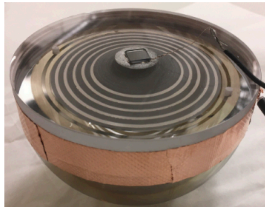
Hybrid photosensor: ABALONE; left (DARWIN R&D with SiPM); right: NIM 954, 2020
