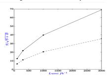
▶ Data are produced at  $\sqrt{s} = 13$  TeV and the points correspond to an integrated luminosity of 100, 300, 1000 and 3000 fb<sup>-1</sup>. Notice that event rates are computed after implementing the acceptance cuts.
