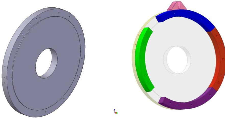
Can we have the upstream (420mm) and downstream (600mm) Virostek plate CAD models? We are interested in the mounting holes for the TOF cage split rings, the supporting brackets, and lifting points.
