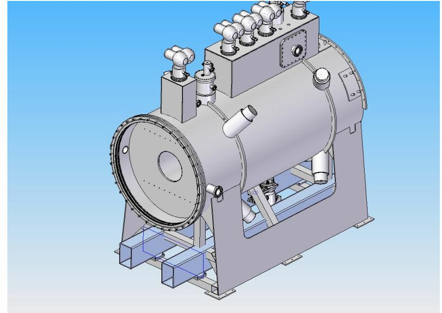
Currently there is a clash between the Spectrometer Solenoid support frame and the restraint beams.
