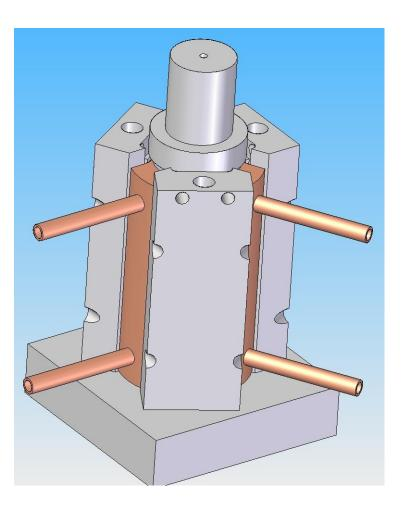
Once the assembly has passed all the QA requirements it is to be potted. A potting jig has been designed and manufactured from PTFE
