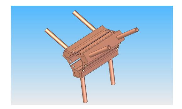
The cooling was revisited and a new cooling jacket designed. This will hopefully make contact with the top outer radius of the coils. The flow of coolant has also been greatly increased. It is hoped that this will aid performance improvement as the cooler the coils run the less resistance and so more power can be fed in. The cooling jacket segments are being manufactured at Imperial College and will be vacuum brazed the tested.
