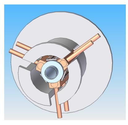
Once the assembly is potted and passed further QA it is to be installed into a modified version of the original body, this has 2 extra slots to accommodate the cooling pipes and welded into position.
